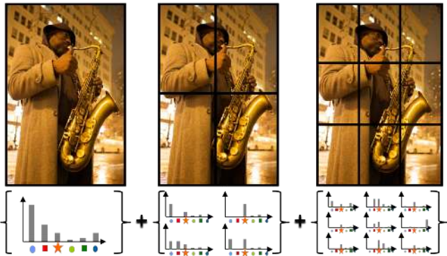
Fig. 2 We apply a three level pyramid on the bounding boxes of the action recognition datasets. Separate BOW histograms are constructed for each cell and are concatenated to form the final action descriptor. In this paper we use a pyramid representation with three levels, yielding a total of 14 cells.
