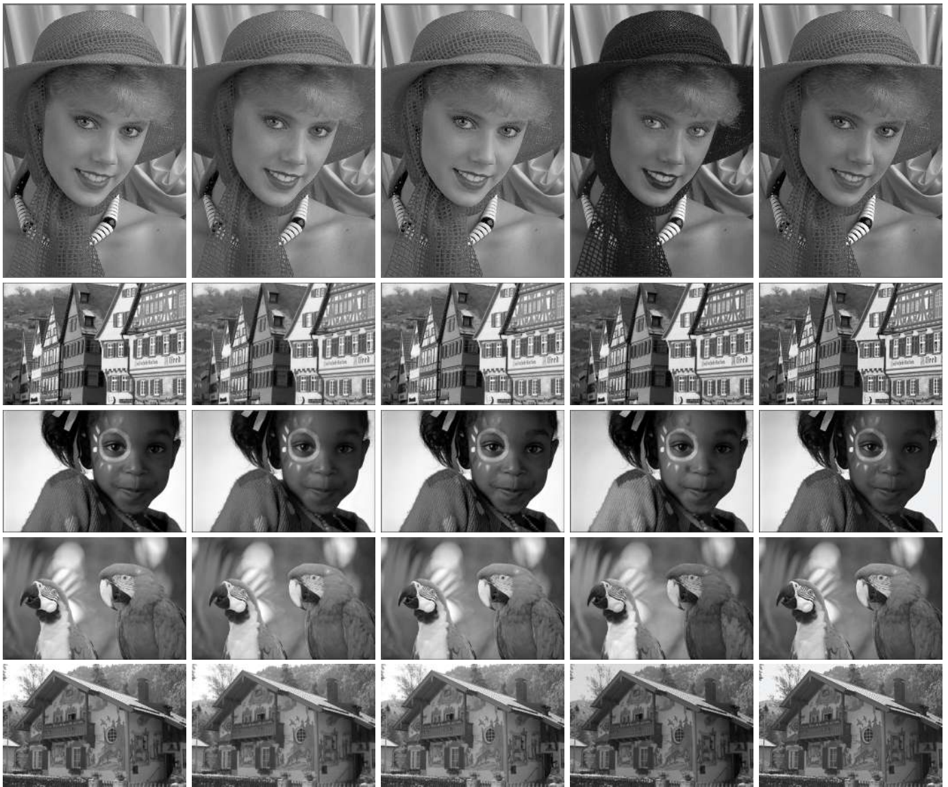
Fig. 2. Resulting greyscale images for the Kodak test images shown in Figure 1. Left to right: CIELAB L^* , \Delta E_{00} , \Delta E_{99} , Du, and Smith.
