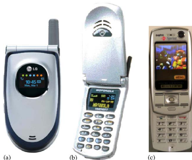
Fig. 14. Pictures of some cell phones equipped with OLED displays: LG VX4600 (a), Motorola Timeport P8767 (b), Sanyo Sprint (c).
