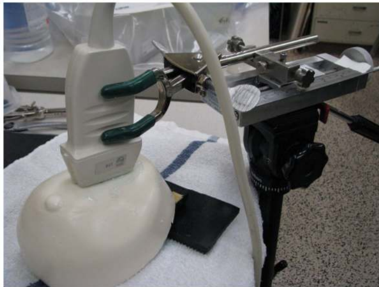
Figure 11. A CIRS breast elastography phantom was imaged using CUSE. The ultrasound transducer was mounted on a mechanical stage. By translating the transducer, the inspected inclusion will change its relative position to the transducer.
