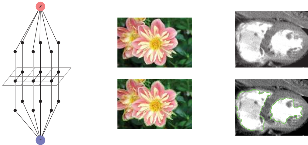
Figure 8. Example of graph construction to incorporate unary terms for unsupervised segmentation. Each node is connected to a source node and sink node through an intermediary node which is weighted to reflect the strength of the positive and negative unary terms. This construction is then applied with a simple appearance prior to automatically segment two images.
