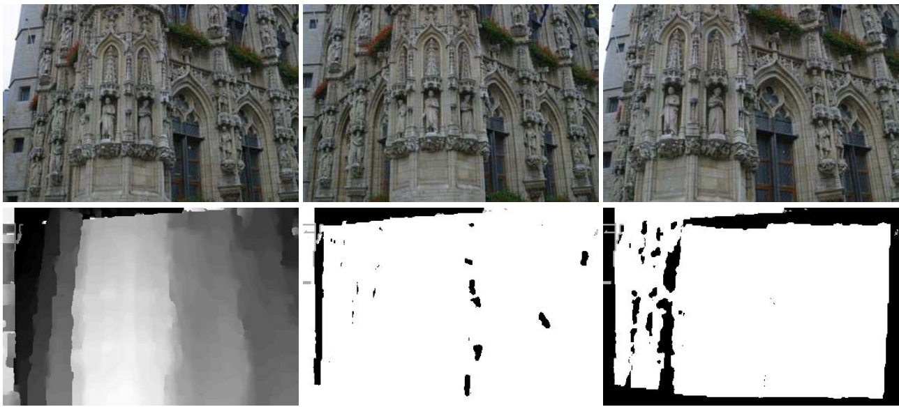
Figure 5. Cityhall scene. Top: the three input images, the camera position of ideal image y^* was chosen to be the left image. Bottom: estimated depth and visibility.
