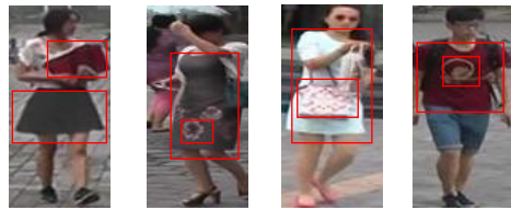
Figure 1. Note that paired salient objects of different sizes can be commonly found in pedestrian images. Our CBlock is designed to explicitly learn such combined patterns.
