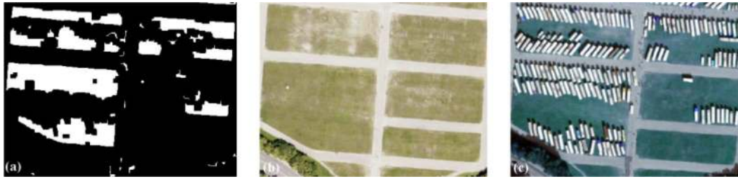
Fig. 19. Subset of the area in Munich: (a) Result of change detection (black: no change, white: change), (b) image taken before the Oktoberfest and (c) image taken during the Oktoberfest.
