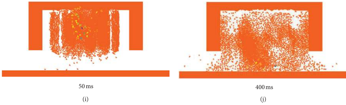
FIGURE 12: Stress wave propagation and rock failure process of the sublevel caving by blast (B-B cross profile). (a) 0.2 ms, (b) 0.4 ms, (c) 0.6 ms, (d) 0.8 ms, (e) 1 ms, (f) 1.2 ms, (g) 24 ms, (h) 26 ms, (i) 50 ms, and (j) 400 ms.
