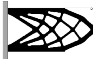
Fig. 3: Design optimized with length scale control; without overhang angle control, c = 1644 , M_{\text{nd}} = 4.50\% .
