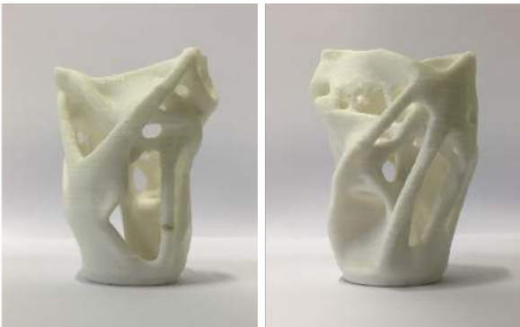
Fig. 23: Different views of the printed tensegrity joint with a bottom-to-top building direction; no additional support structure has been used.
