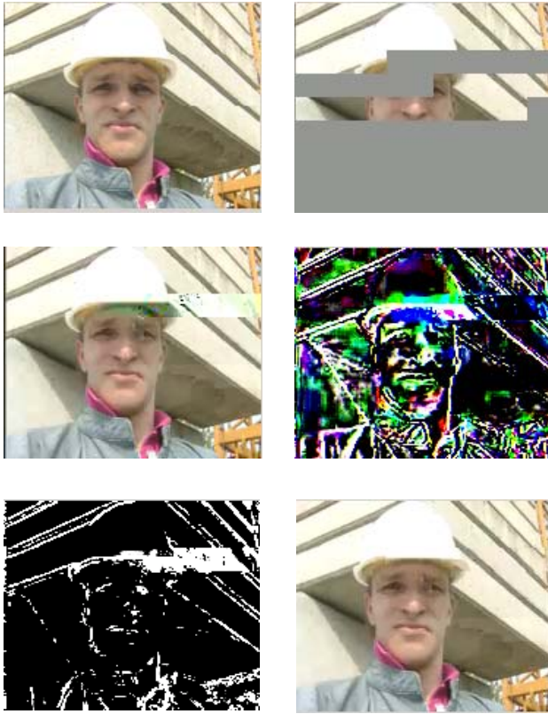
Fig. 1. Example of sequential decoding and error concealment: original picture, picture with lost slices (packets), picture with residual errors after sequential decoding, difference picture, artifact detection metric, picture after concealment.
