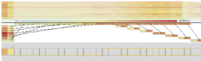
Fig. 6: Logical (top) and Cluster (middle/bottom) view of a merge tree gather, further discussed in Section 5.1. The bottom row shows the unopened root of the cluster hierarchy, summarizing the events in the cluster: many processes active in the first two steps, few in the rest. Above the cluster are individual timelines showing the communication neighborhood of one process of interest. The focus processes show structure which can no longer be seen in the logical view.
