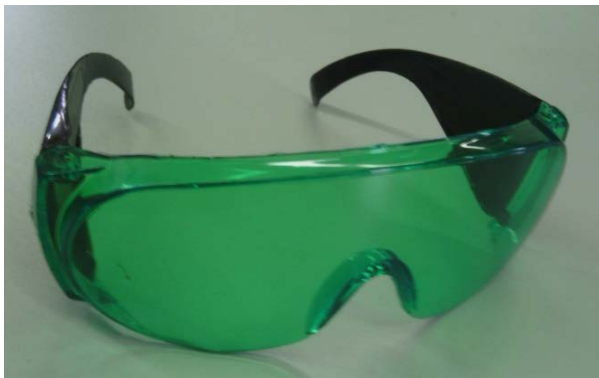
Figure 7: Safety glasses made in the integrated process of additive manufacturing technology and vacuum casting
