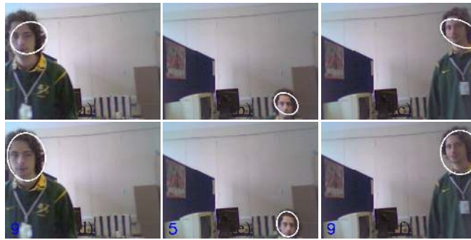
Figure 8: Examples of tracking results (Target F1, frames 85, 364, 1120) using colour histograms (top row), and adaptive colour and orientation histograms (bottom row).
