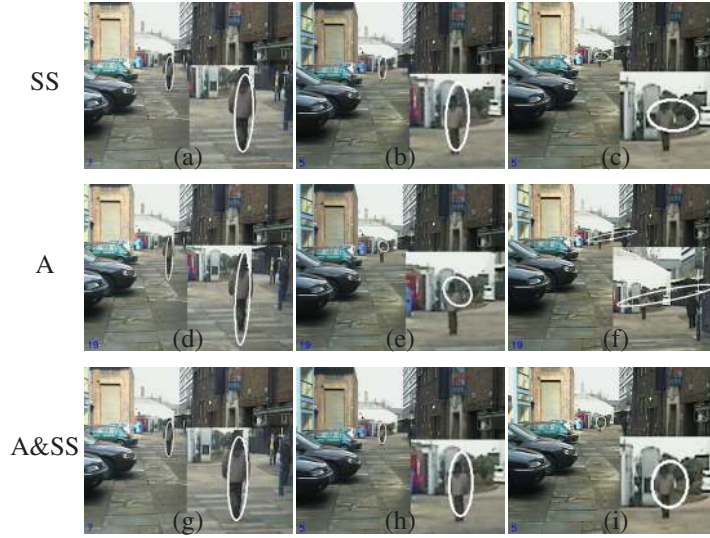
Figure 6: Examples of tracking results (Target P3 frames 160, 465, 659) using automatic scale selection (SS), adaptive weighting for Particle Filter (A), and both (A&SS).
