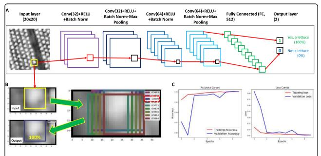
**Fig. 4 A CNN-based learning architecture established for lettuce counting. a** The architecture of the trained CNN model, which generates a binary output representing the probability of whether a yellow bounding box contains a lettuce signal. **b** If the probability is close to 100%, it indicates that it is highly likely that the bounding box encloses a whole lettuce. **c** The training and validation accuracy and loss curves of the model
