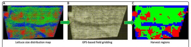
Fig. 6 A GPS-based harvest map based on lettuce size classification. a A colour-coded lettuce size distribution map (small is coloured blue, medium is coloured green, and large is coloured red). b The field is segmented into thousands of grids based on the optimal GPS resolution. c Grids are coloured with the most representative lettuce size category across the image, representing harvest regions of the whole field
