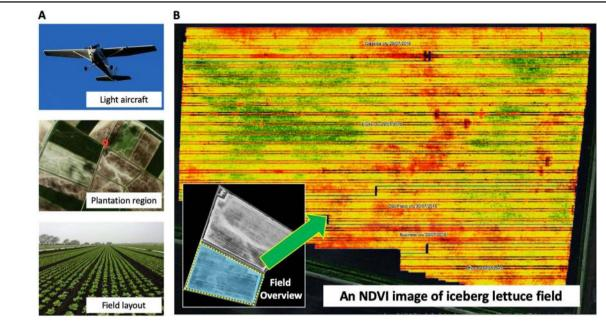
Fig. 1 Ultra-scale NDVI aerial imaging accomplished routinely through a fixed-wing light aircraft operated by G's Growers. a The flying route and aerial imaging were designed to facilitate cross-site crop layout assessment and yield prediction. b A series of ultra-large NDVI images at 3 cm GSD spatial resolution were acquired to record 0.8–1.6 million lettuce heads per field, at H1 and H2 stages
