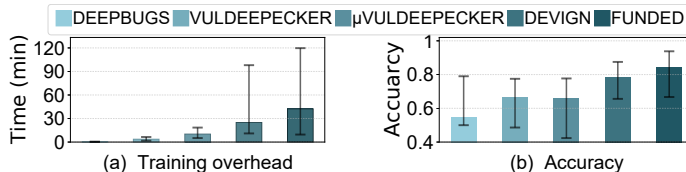
Fig. 19. Training overhead (a) and accuracy (b). The min-max bars show the variances across evaluation settings.
