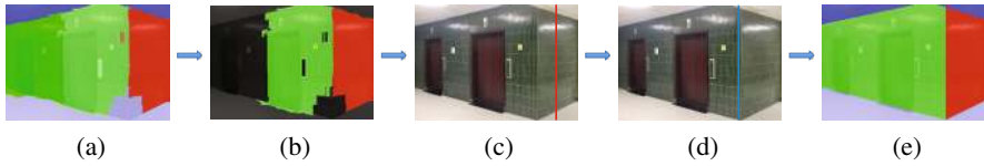
Fig. 6. Continuous optimization: (a) shows the result from discrete optimization; (b) highlights two regions that after the discrete step are labeled with the correct normals, but incorrect depths such that they are not connected (at the apparent intersection in the image); (c) shows the 2D projection of the line of intersection of planes represented by the highlighted regions (in red); (d) shows the target line of intersection which obeys image cues (in blue); (e) shows the final result, after the continuous optimization and refining the segmentation
