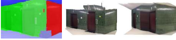
Fig. 5. Result of the discrete optimization. The discrete optimization stage assigns the correct normal, but it fails to distinguish between two parallel planes at different depths splitting the left wall into two regions (as shown by the two different shades of green) at different depths.
