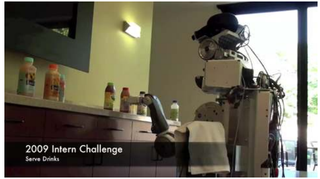
Fig. 5. Implementing a grasping task as part of a larger system task of serving drinks at a restaurant
