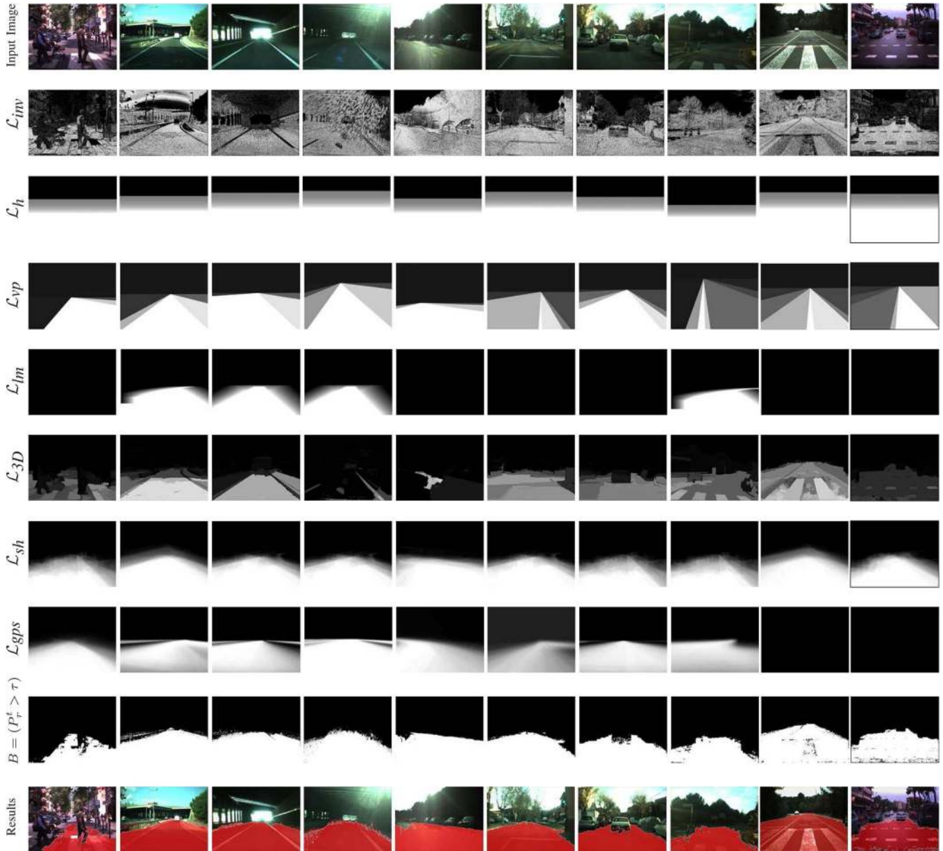
Fig. 13. Example road detection results using cues and priors. From top to bottom: input image; color-based cue \mathcal{L}_{inv} ; horizon line \mathcal{L}_h ; vanishing point \mathcal{L}_{vp} ; lane markings \mathcal{L}_{lm} ; 3-D scene layout \mathcal{L}_{3D} ; road shape \mathcal{L}_{sh} ; online prior \mathcal{L}_{gps} ; final road mask B ; and the road mask overlapped on the input image.
