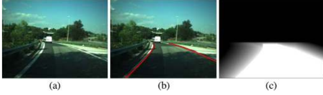
Fig. 9. (a) Original image. (b) Detected lane markings overlapped on the input image. (c) Road confidence map estimated from lane marking results. The whiter the pixels, the higher the pixel potential of being a road pixel.
