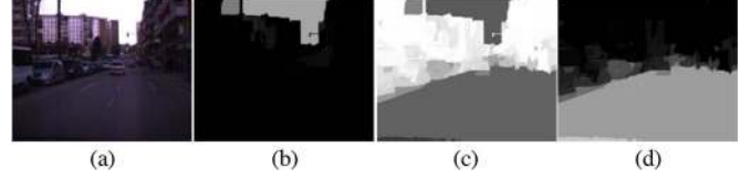
Fig. 10. (a) Input image is partitioned in three 3-D geometry classes: sky, vertical surface and ground. Using the approach of Hoiem et al. [27], a pixelwise confidence is estimated for each class [(b) sky areas P_s , (c) vertical surfaces P_v , and (d) ground areas P_g ]. The whiter the pixels, the higher the potential of a class.
