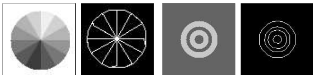
Figure 1: a. First synthetic image containing various object edge orientations. b. Segmentation result.
