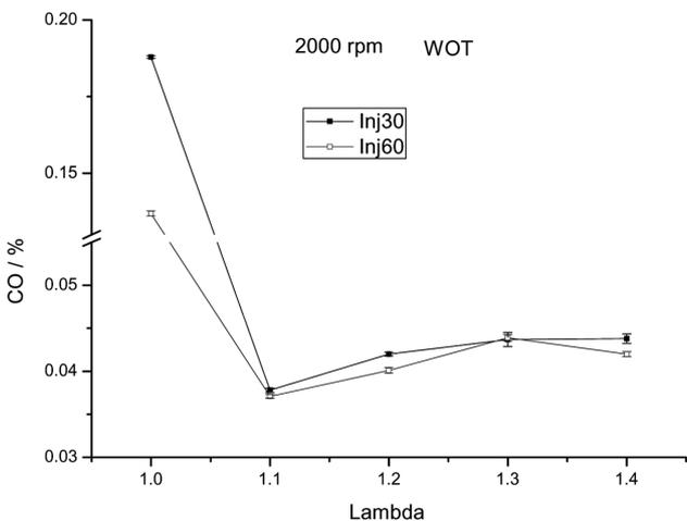
Fig. 9. Engine-out CO emissions versus lambda at MBT spark timing under different operating conditions.
