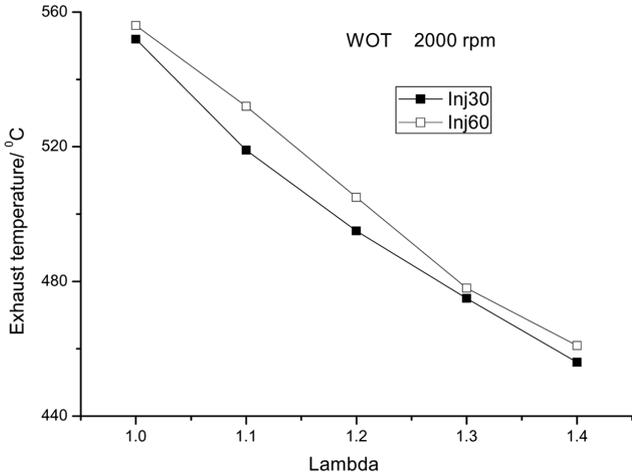
Fig. 8. Exhaust temperature versus lambda at MBT spark timing under different operating conditions.
