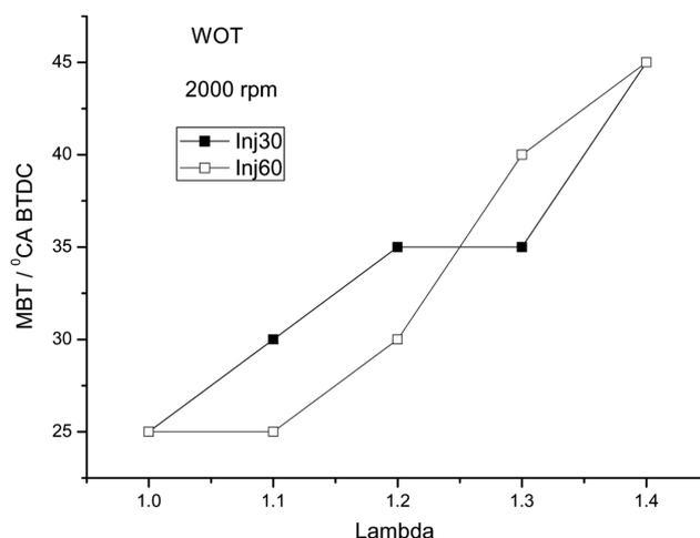
Fig. 2. MBT spark timing versus lambda under different operating conditions.
