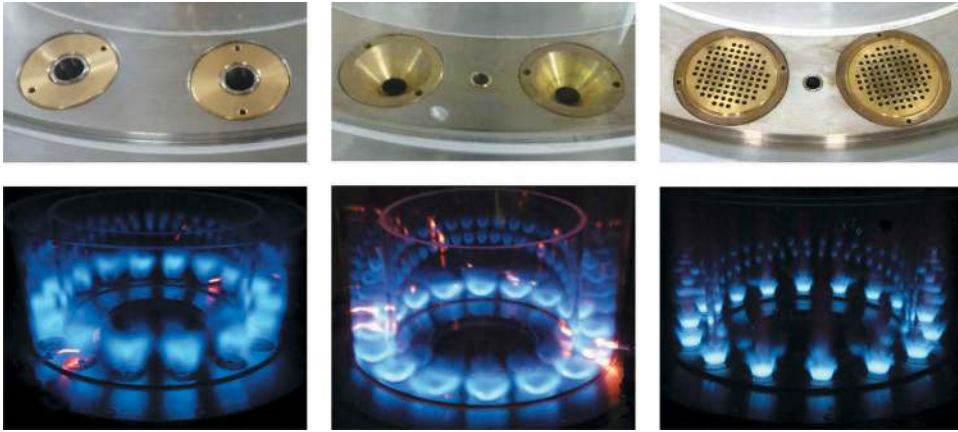
Figure 2. Injector geometry and induced flame shape in the annular setup. Left: MICCA, the injectors feature a swirler and a cylindrical exhaust channel. This configuration is used in the light-round investigation. Center: MICCA2, the injectors feature a swirler and a conical cup. This geometry is used in the thermo-acoustics instability investigations. Right: MICCA3 with matrix injectors used to examine thermo-acoustics instabilities in an environment which features low levels of random perturbations.
