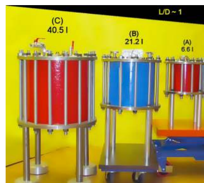
Fig. 1. Calorimeters: A ( V=6.6 liters: L=21 cm, D=20 cm, L/D=1.05 ), B ( V=21.2 liters: L=30 cm, D=30 cm, L/D=1.00 ) and C ( V=40.5 liters: L=37.9 cm, D=36.9 cm, L/D=1.03 ).
