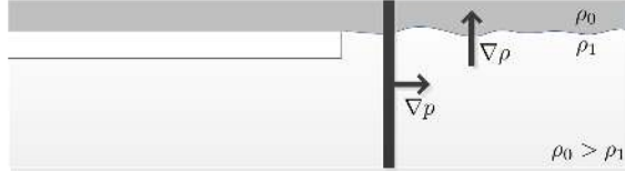
Figure 5: Shear layer showing the dense fuel against the wall and the less dense oxidizer in the core.
