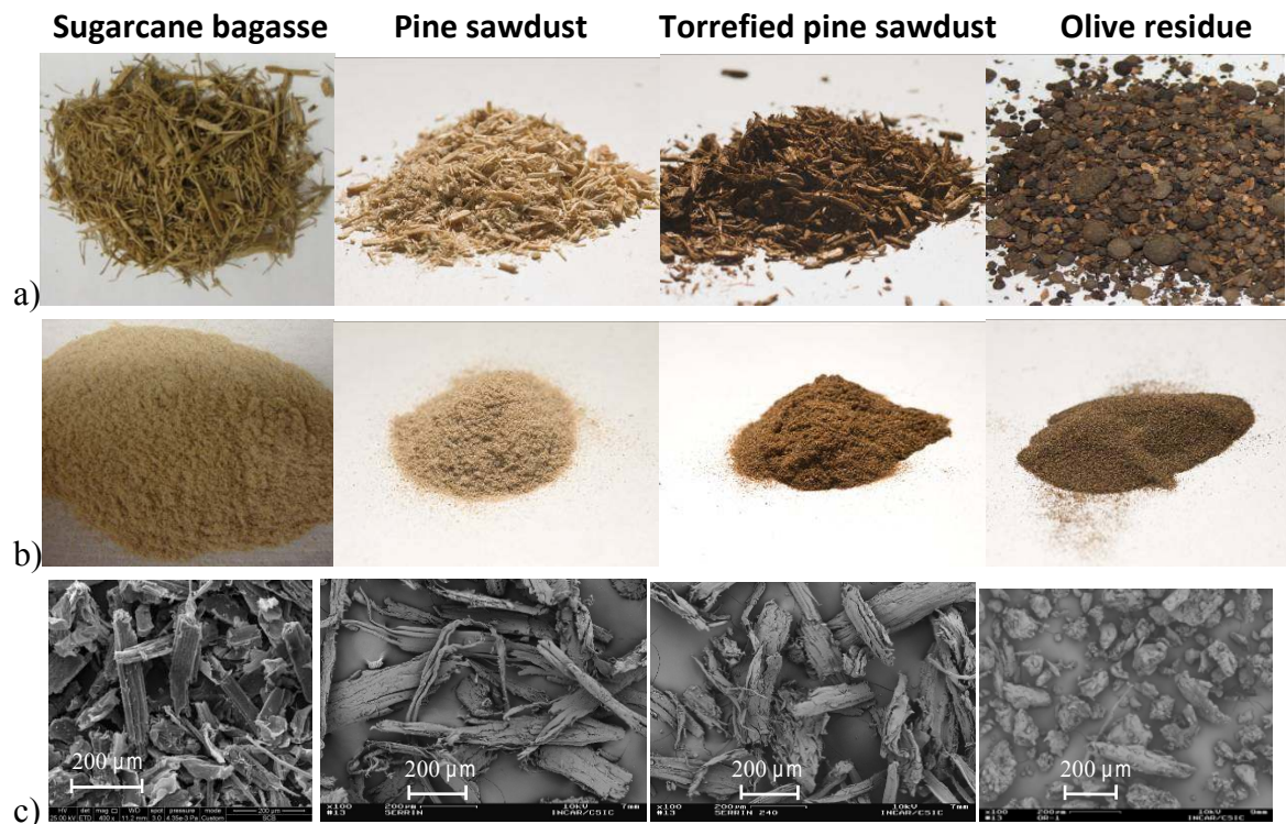
Figure 1. Physical appearance of the biomasses residue; (a) original biomasses, as received, (b) ground and sieved, (c) SEM micrographs detailing individual particles.
