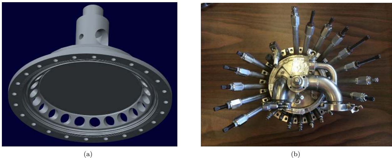
Figure 4. Morpheus main engine injector acoustic cavity layout. (a) Acoustic cavity ring at 45 deg to faceplate. (b) Tunable acoustic cavity configuration.
