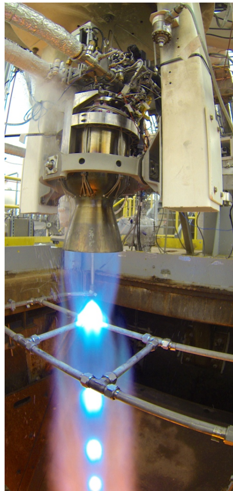
Figure 2. Morpheus Main Engine Testing at SSC test stand E-3, with nozzle exit and flame trench inlet in close proximity.
