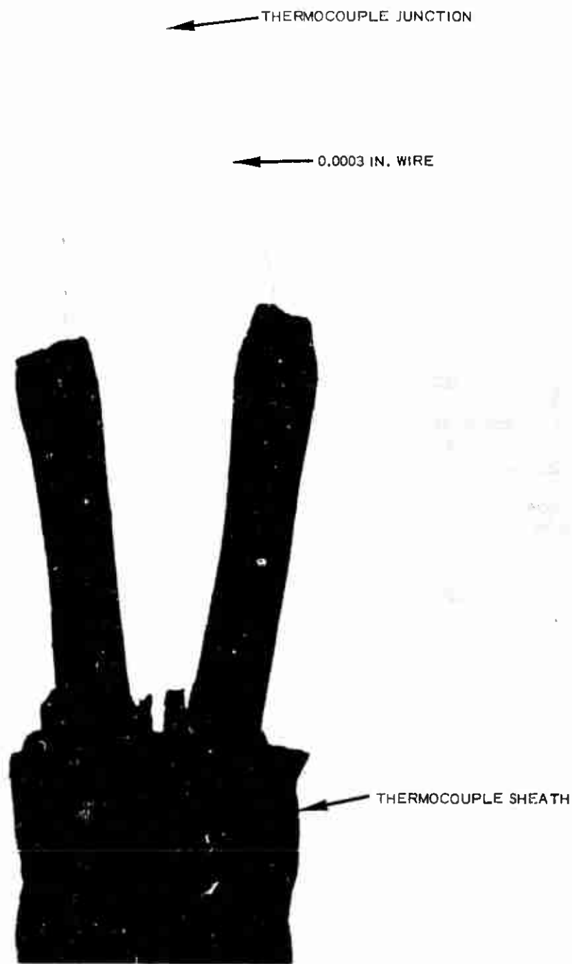
Figure 19 Photomicrograph of Fine-Wire Thermocouple
