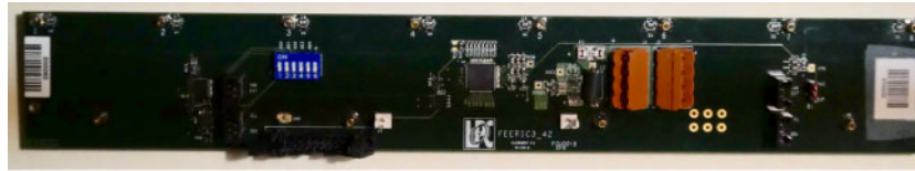
Fig. 78. A front-end board, developed for ALICE, housing the FEERIC ASIC in the center of the board. At the top, the eight pins connecting the readout strips (designed for 4.5 cm readout strips in this case) are visible. The four pins on the bottom of the picture are for grounding. The board shown is 32.5 cm long and 5 cm wide, but the final dimensions will be determined by the optimal BS-CRV segmentation.
