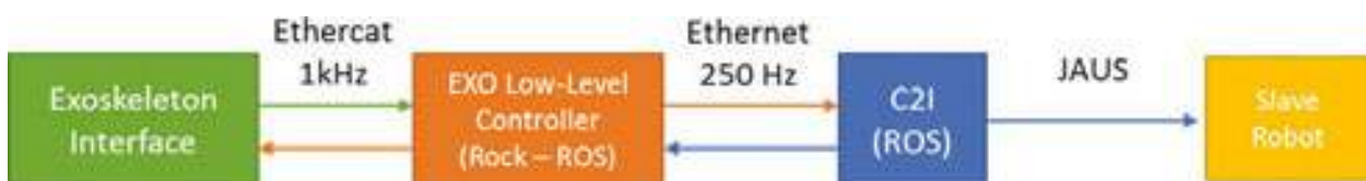
Figure 27. Exoskeleton control architecture (source: ICARUS).
