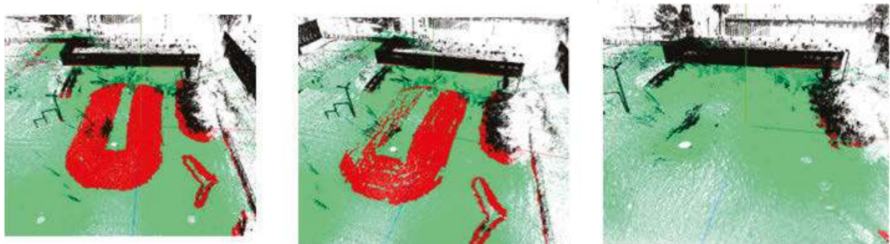
Figure 37. The traversability analysis: traversability for UGV with 10° max slope, 18° max slope and 44° max slope (source: ICARUS).
