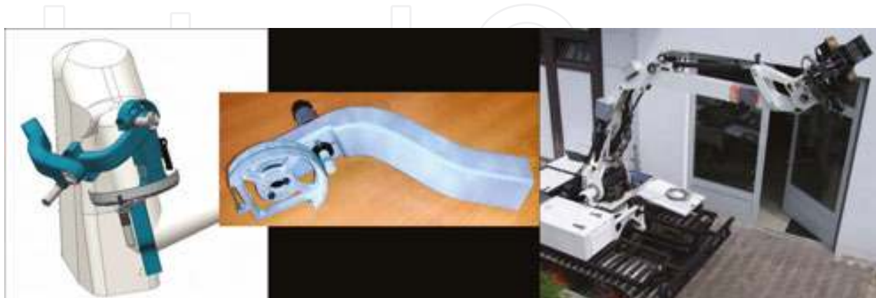
Figure 29. (i) SAM exoskeleton upper part advanced design and rapid prototyping part integration test. (ii) LUGV with extended manipulator (source: ICARUS).
