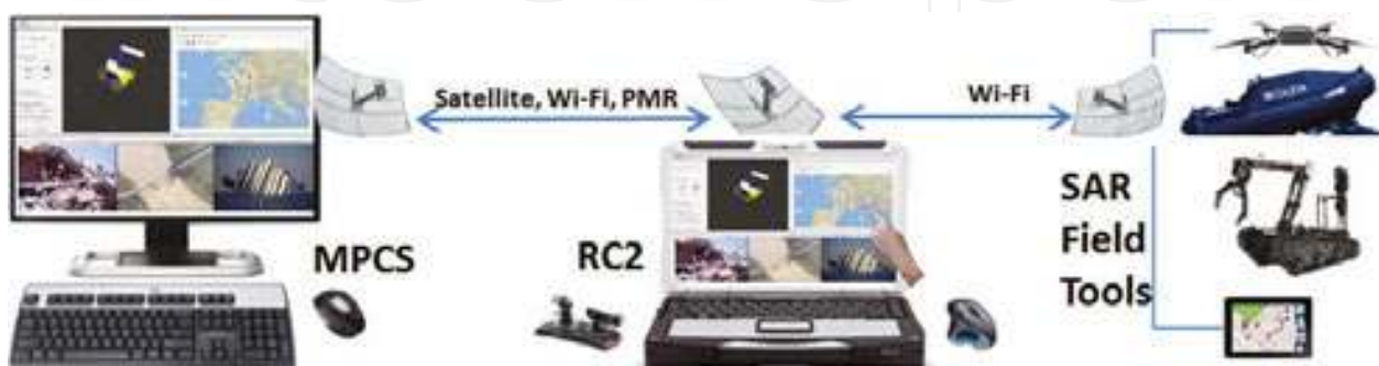
Figure 1. C2I deployment and communication framework (source: ICARUS).
