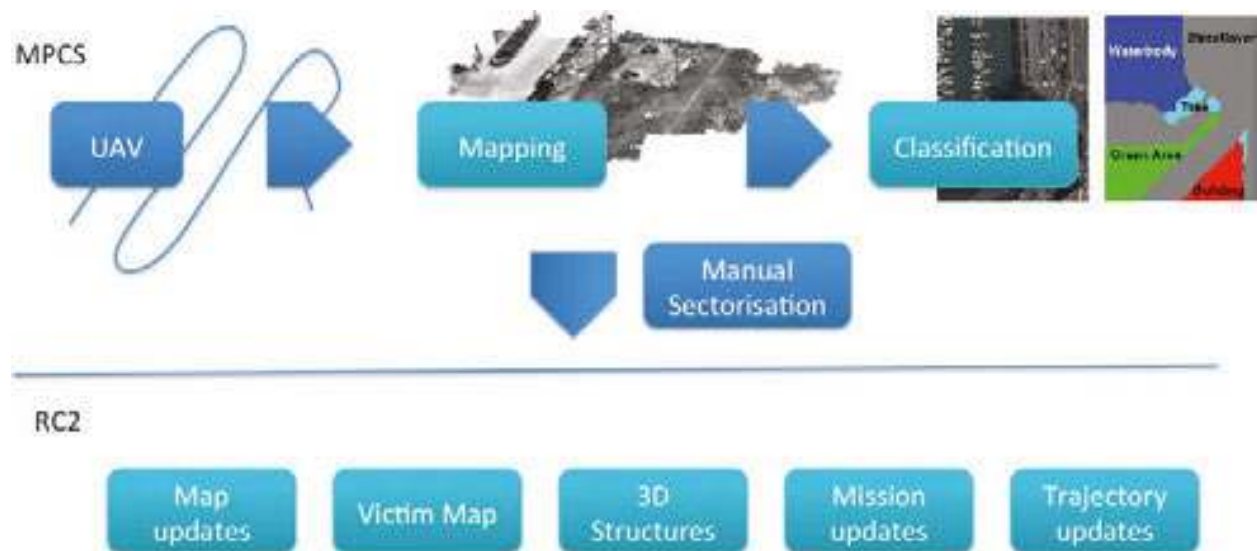
Figure 13. Concept of operations with data fusion functionalities (source: ICARUS).
