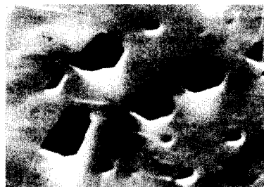
FIG. 2. Scanning electron micrograph of intergranular vacancy pits in a 99.99% Al specimen after same heat treatment as Fig. 1 (grain boundary separated by liquid-gallium decohesion) ( \times 5000 ).
