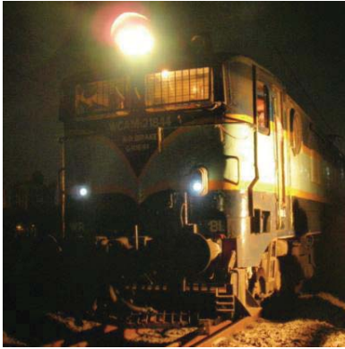
Fig. 10. Locomotives for load testing (design train) that is made available for the tests carried out.
