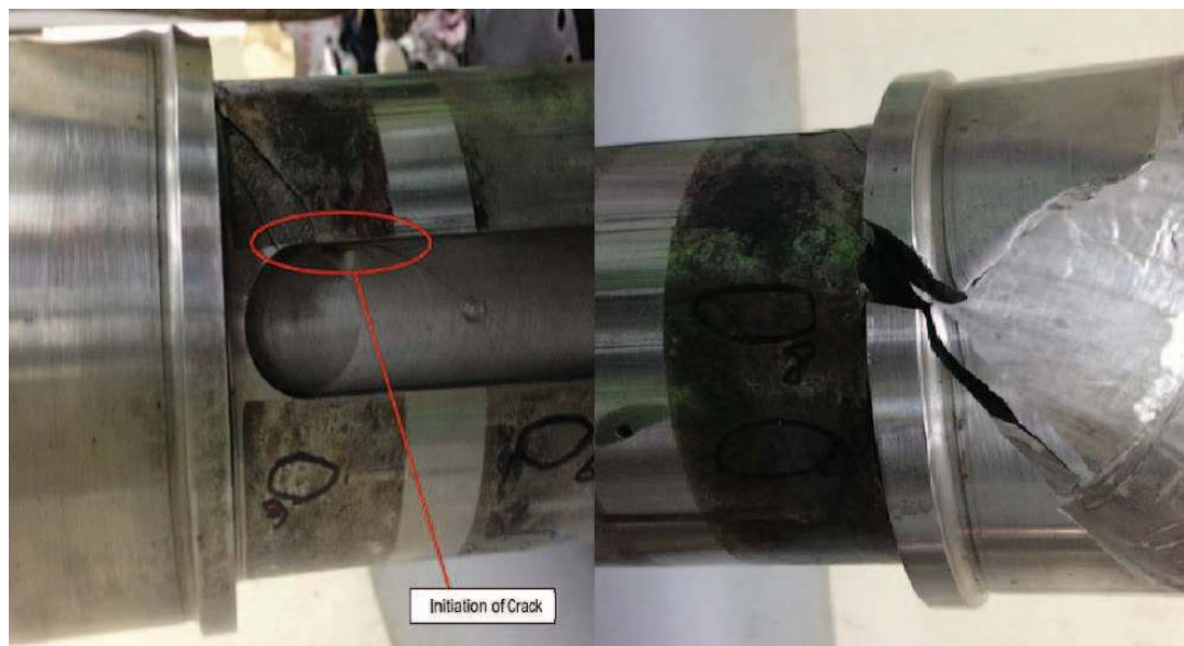
Figure 3 The Characteristic Torsional Failure Crack Shape [8]
