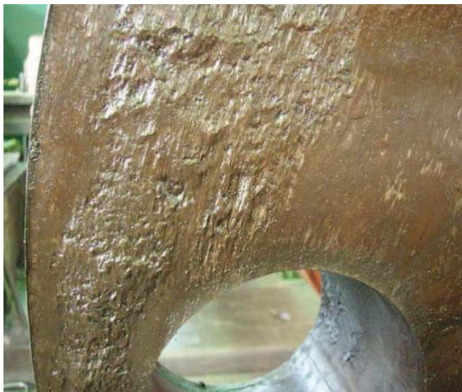
Figure 6 Fatigue Indicative Fretting on Surfaces [13]
