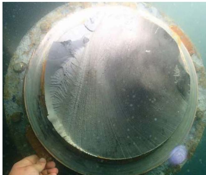
Figure 7 Uniaxial Fatigue Failure Crack Shape [15]
