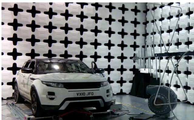
Fig. 6. Electric field measuring with log-periodic antenna
