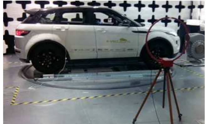
Fig. 7. Magnetic field measuring with loop antenna
