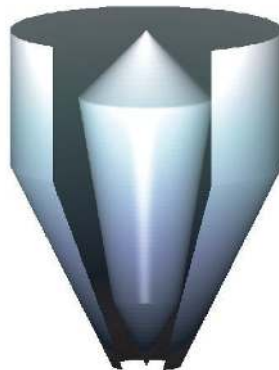
Fig. B.1 Cutaway view of a bin with a flow correction insert.
