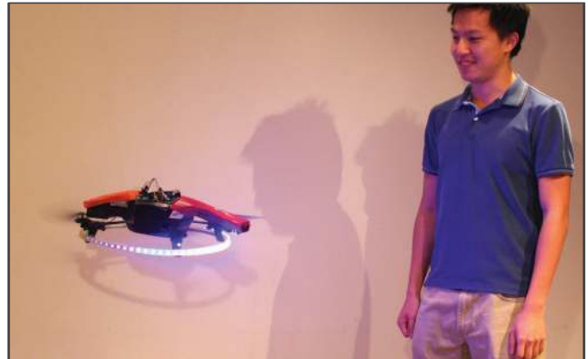
Figure 1: We explore the design of visual signaling mechanisms for flying robots to support the expression of robot intent and increase usability in colocated interactions.
