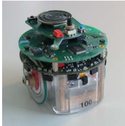
Fig. 2. The e-Puck: a small-scale robotic platform for education. Shown here with the radio communication board stacked between the basic module and the jumper board.
