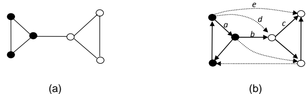
Fig. 2. (a) A graph consisting of two communities. (b) Adding semantics to the edges could lead to disappearing of the two communities since new link d could be derived out if semantic links a and b satisfy rule a-b \Rightarrow d . A new semantic link e could be further derived from d and the existing semantic link c .
