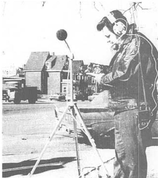
Figure D-4. Microphone System Being Assembled by TSC Technician
