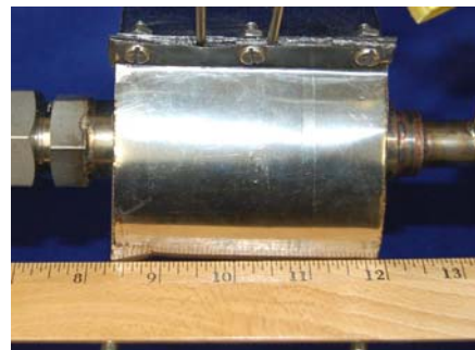
Figure 3. Photo of the Sabatier reactor prototype developed at PCI.
