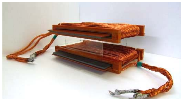
Fig. 6. Photograph of 1.5 kW transformer
