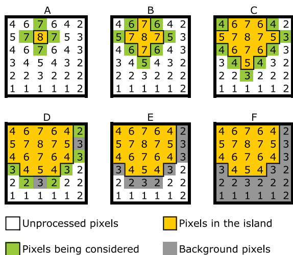
Figure 1. A demonstration of the operation of the FLOODFILL algorithm. The small ‘image’ has pixel values that are in units of the background noise. The seed threshold is \sigma_s = 5 and the flood threshold \sigma_f = 4 . The orange pixels are those that have been assigned to an island, green pixels are those that are being considered, grey pixels have been rejected and white pixels are yet to be considered. In panel (A) the brightest pixels is used to seed an island. Pixels adjacent to the island are then inspected (coloured green). In panel (B) the pixels under consideration are brighter than the flooding threshold and are added to the island. The process is repeated in panels (C) and (D). In panel (E) there are no more pixels adjacent to the island that have not been inspected. In panel (F) all pixels have either been assigned to an island (orange) or are labelled as background (grey).
