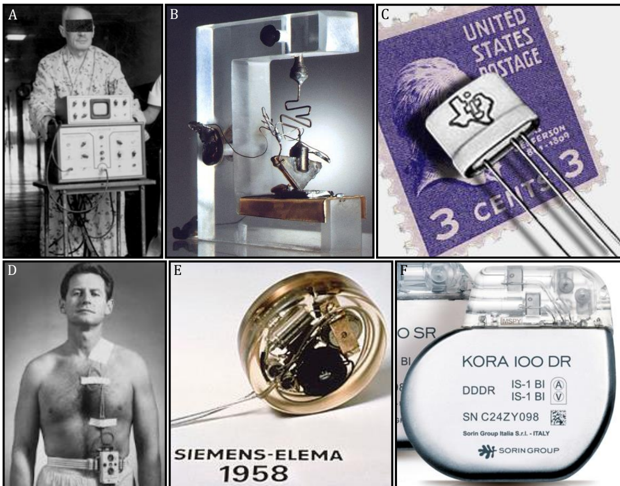
Figure 2.1: Evolution of implantable cardiac device. A) External portable pacemaker powered through extension cord. [104] B) Modern replica of the world's first germanium contact point transistor. (Image courtesy of Alcatel-Lucent USA, Inc., Bells laboratory) C) The first commercially available transistor presented by Texas Instruments in front of the 3 cent postage mark. (Image courtesy of Texas Instruments Inc.) D) Programmable battery-operating wearable and portable cardiac pacemaker. [110] E) Modern replica of the first completely implantable pacemaker. (Image courtesy of Wikipedia) F) State of the art of the MRI compatible implantable pacemaker. (Image courtesy of Sorin group)
