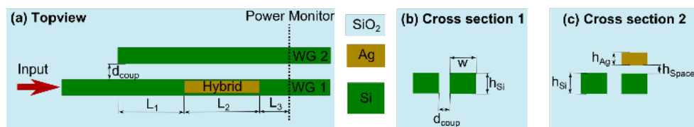
Fig. 1. (a) Top view of the broadband directional coupler (b) Cross section of the first and third silicon coupler sections. (c) Cross section of the second section. Positions of power monitors used in finite difference time domain (FDTD) simulation for calculating of power in the output waveguides are shown by dashed lines.
