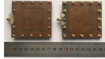
Fig. 2 Photograph of the fabricated dual-cavity SIW-based filtenna. Left: top view. Right: bottom view.
