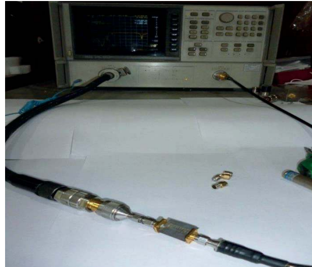
Figure 13. The measurement workbench with an HP8720B network analyzer.
