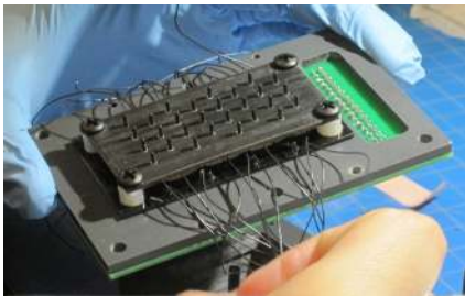
Figure 6: Photograph of 28-element tactile array during assembly.
