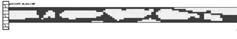
Figure 12. Optimal structure on the 100 \times 10 mesh for 10 \times 1 cantilever plate for the Voronoi representation. D_{lim} = 12 , number of cells = 105, weight = 0.479. CPU time = 14 s/gen.
