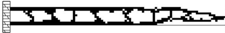
Figure 13. Optimal structure on the 100 \times 10 mesh for 10 \times 1 cantilever plate for the Voronoi-bar representation. D_{lim} = 12 , number of cells = 91, weight = 0.424. CPU time = 14 s/gen.
