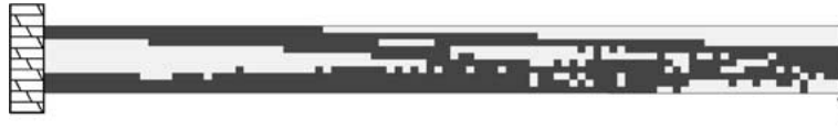
Figure 17. Optimal structure on the 100 \times 10 mesh for 10 \times 1 cantilever plate for the IFS representation. D_{lim} = 12 . weight = 0.58. CPU time = 15 s/gen.
