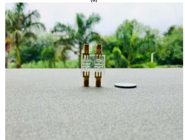
FIGURE 10. Fabricated 4 element MIMO antenna (a) Top View (b) Front View.
