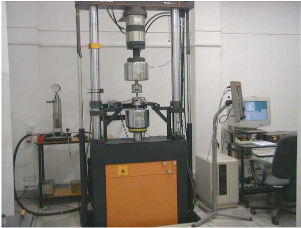
Figure 4. Servo-hydraulic testing machine INSTRON® 1343
