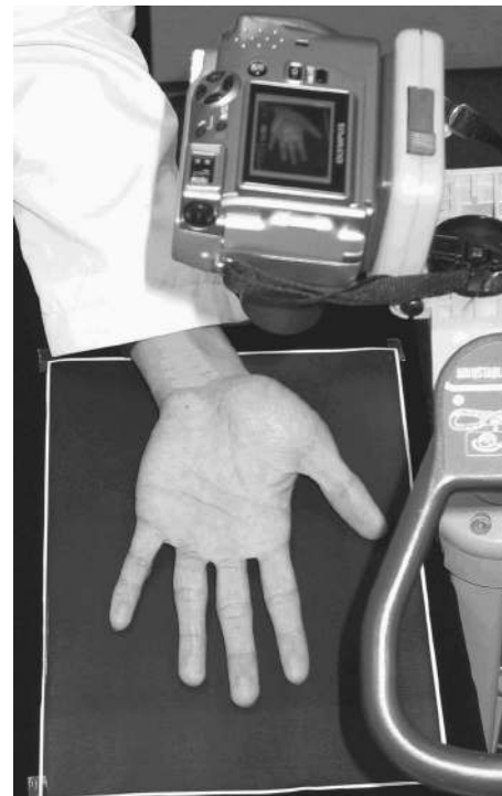
Fig. 7 Hand shape and palm acquisition device of Kumar et al. (from Refs. 21 and 22).
