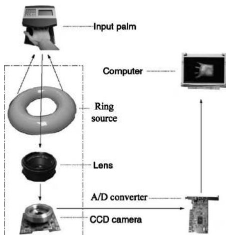
Fig. 6 Palmpoint capture device (from Ref. 43).
