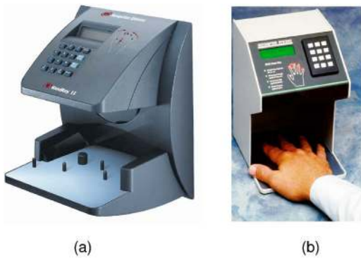
Fig. 5 (a) Handkey II, (b) ID3D Handkey, the commercial hand geometry-based verification devices from Schlage Recognition Systems.
